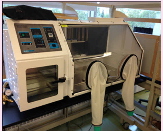
The Anaerobic Chamber is used to grow microbes without oxygen.
