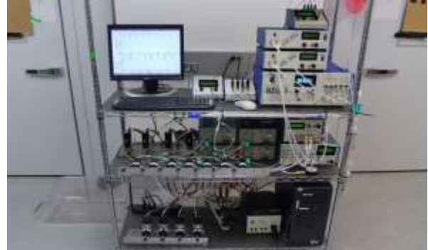
Fig. 6 A fully automated respirometry system located in the Integrated Sciences Building at UAA.
