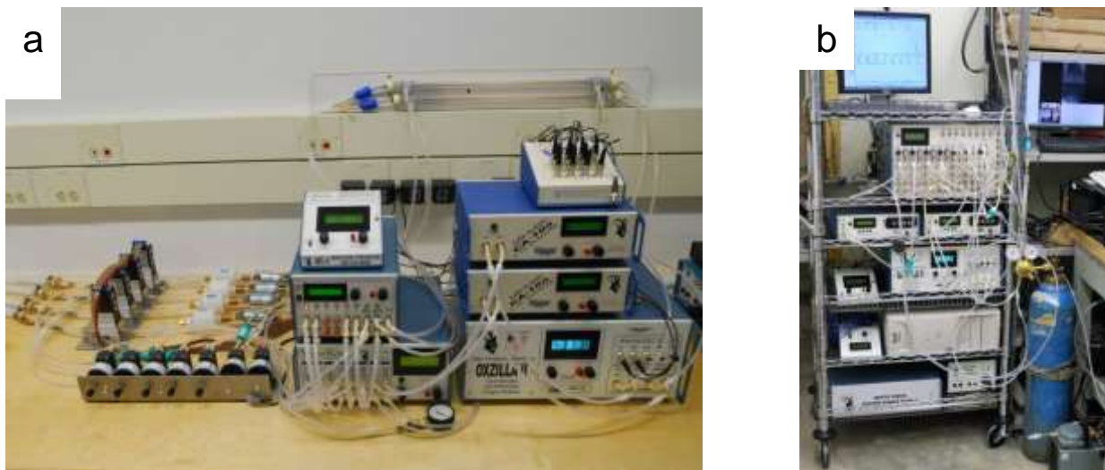
Fig. 5. Fully automated respirometry systems in the bear (a) hibernation facility and (b) summer holding facility.
