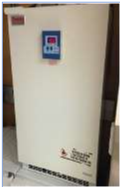
Figure 2: Incubators are used to maintain the optimal growth temperature. The AIMS Core has five incubators with a temperature range of 4-75°C and two shaking incubators with a temperature range of 4-65°C.
