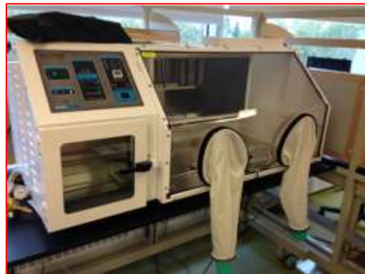
Figure 3: The Bactron anaerobic chamber allows for culturing microbes in oxygen depleted environments similar to the conditions the microbes would be exposed to in the gut. The chamber also contains an incubator to maintain optimal growth temperatures (between room temperature to 55°C) while under anoxic conditions.
