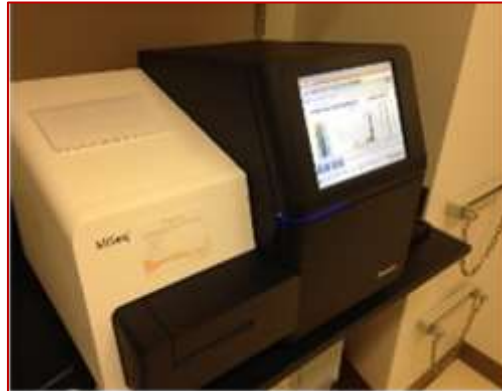
Figure 6: The Illumina MiSeq is next generation sequencing that will produce up to 200 million DNA sequences and can be used to sequence the genome of novel microbial isolates, 16S rRNA genes, or metagenomics/transcriptomics of low diversity communities.
